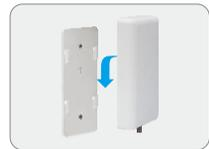
3. Align the antenna with the magnetic clasp and push it down to stick the magnetic clasp, then connect the coaxial line.
