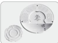
4. Separate the host with the magnetic clasp.
